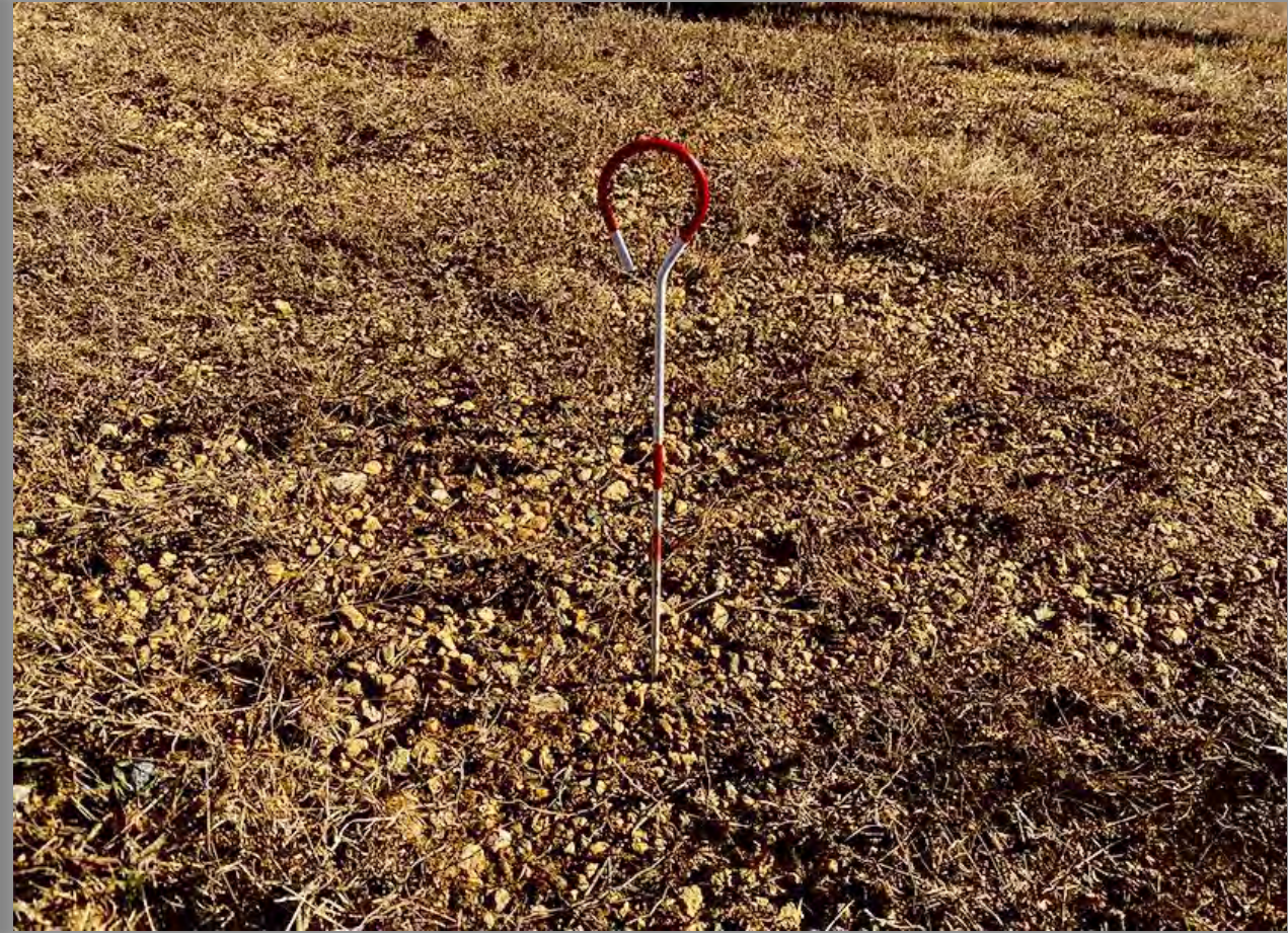
1" Penetration with Survey Pin
